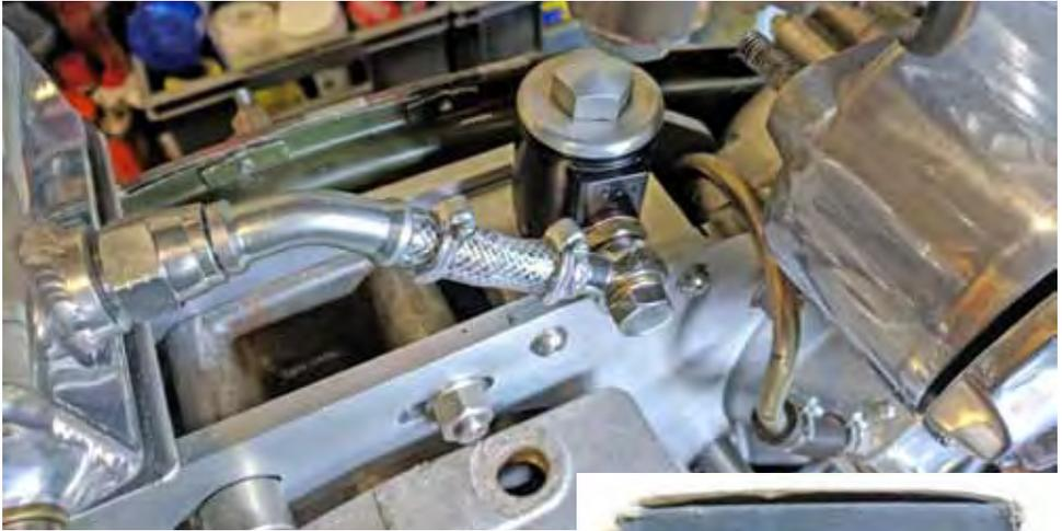
I've been working through multiple solutions to fit a hidden oil filter to a NorVel I'm building. To get the engine and gearbox in the right position, I spaced out the sprocket centres, a by-product of which is I can fix a Triumph/BSA filter in a custom chamber between the engine plates, the U bend acting as a anti drain valve.
